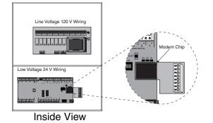
ULTRAVAC™ Controller with Modem Installed
